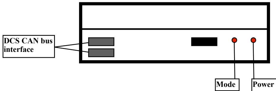
Figure 8. A view of the fan tray with the control interfaces as seen from the front of the crate.
