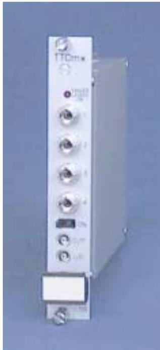
Fig. 10 TTCmx laser transmitter
